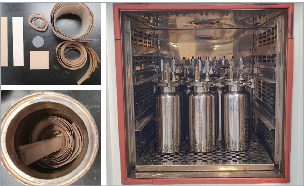
[Fig. 6] A test of insulation oil deterioration characteristics (conducted by Hyosung)
