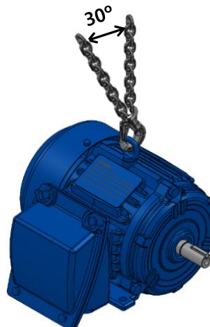
Figure 4.3 - Maximum allowable inclination angle for a motor with only one eyebolt
