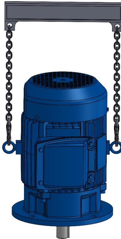
Figure 4.5 - Lifting a vertical type motor
