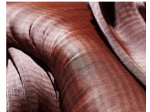
Tire cord made from recycled PET yarn
