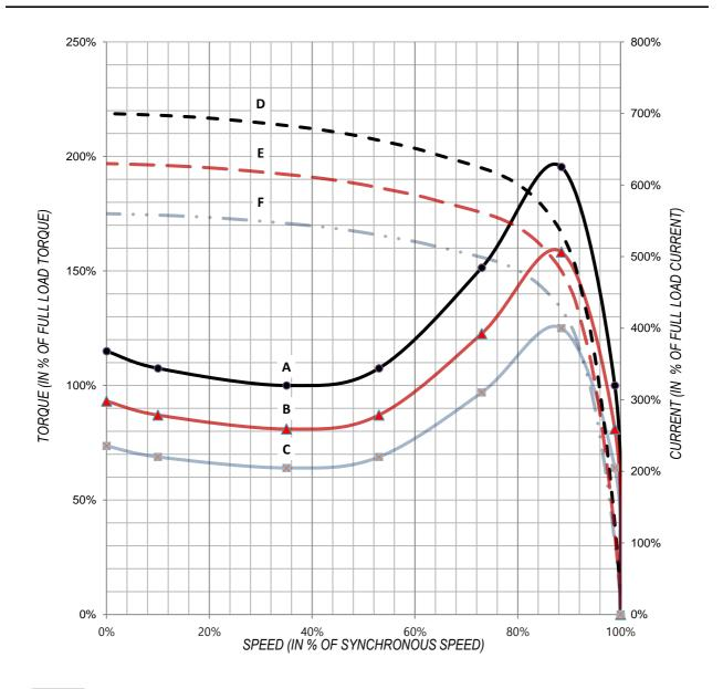
NOTE 100% RATED VOLTAGE : SPEED-TORQUE CURVE AT : SPEED-TORQUE CURVE AT 90% RATED VOLTAGE : SPEED-TORQUE CURVE AT 80% RATED VOLTAGE D : SPEED-CURRENT CURVE AT 100% RATED VOLTAGE : SPEED-CURRENT CURVE AT 90% RATED VOLTAGE : SPEED-CURRENT CURVE AT 80% RATED VOLTAGE
