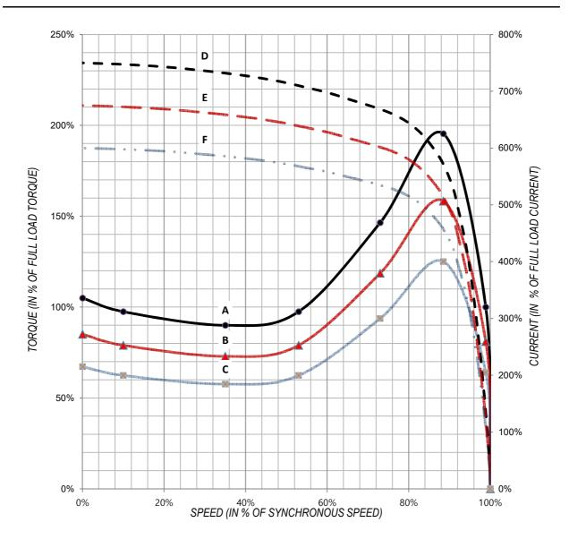
NOTE : SPEED-TORQUE CURVE AT 100% RATED VOLTAGE : SPEED-TORQUE CURVE AT 90% RATED VOLTAGE : SPEED-TORQUE CURVE AT 80% RATED VOLTAGE : SPEED-CURRENT CURVE AT 100% RATED VOLTAGE : SPEED-CURRENT CURVE AT 90% RATED VOLTAGE : SPEED-CURRENT CURVE AT 80% RATED VOLTAGE
