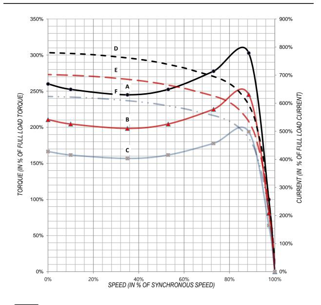
NOTE 100% RATED VOLTAGE : SPEED-TORQUE CURVE AT : SPEED-TORQUE CURVE AT 90% RATED VOLTAGE : SPEED-TORQUE CURVE AT 80% RATED VOLTAGE D : SPEED-CURRENT CURVE AT 100% RATED VOLTAGE : SPEED-CURRENT CURVE AT RATED VOLTAGE 90% : SPEED-CURRENT CURVE AT 80% RATED VOLTAGE
